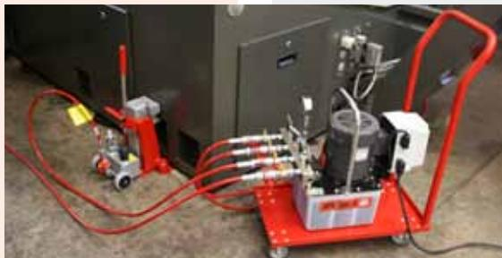
Recommendation: If lifting one side of a load with 2 jacks use electrical pump type JPE, external manual pump JP 26 or air hydraulic pump JPL 15 (see page 15).
